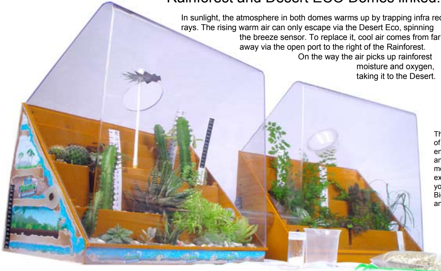
Desert ECO Dome configuration: Roof port open. Left side port closed. Right side port linked to Rainforest ECO Dome
